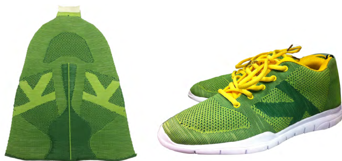
Figure 12. Flat-knitted half-shaped uppers and shoe
